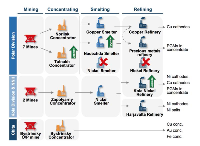
Processing stages of nickel ores at the Norilsk deposit
