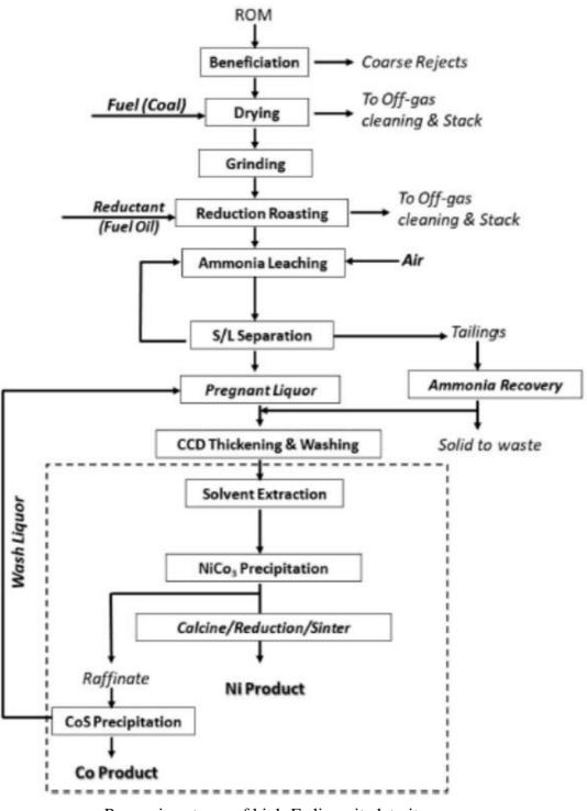
Processing stages of high-Fe limonite laterite ores
