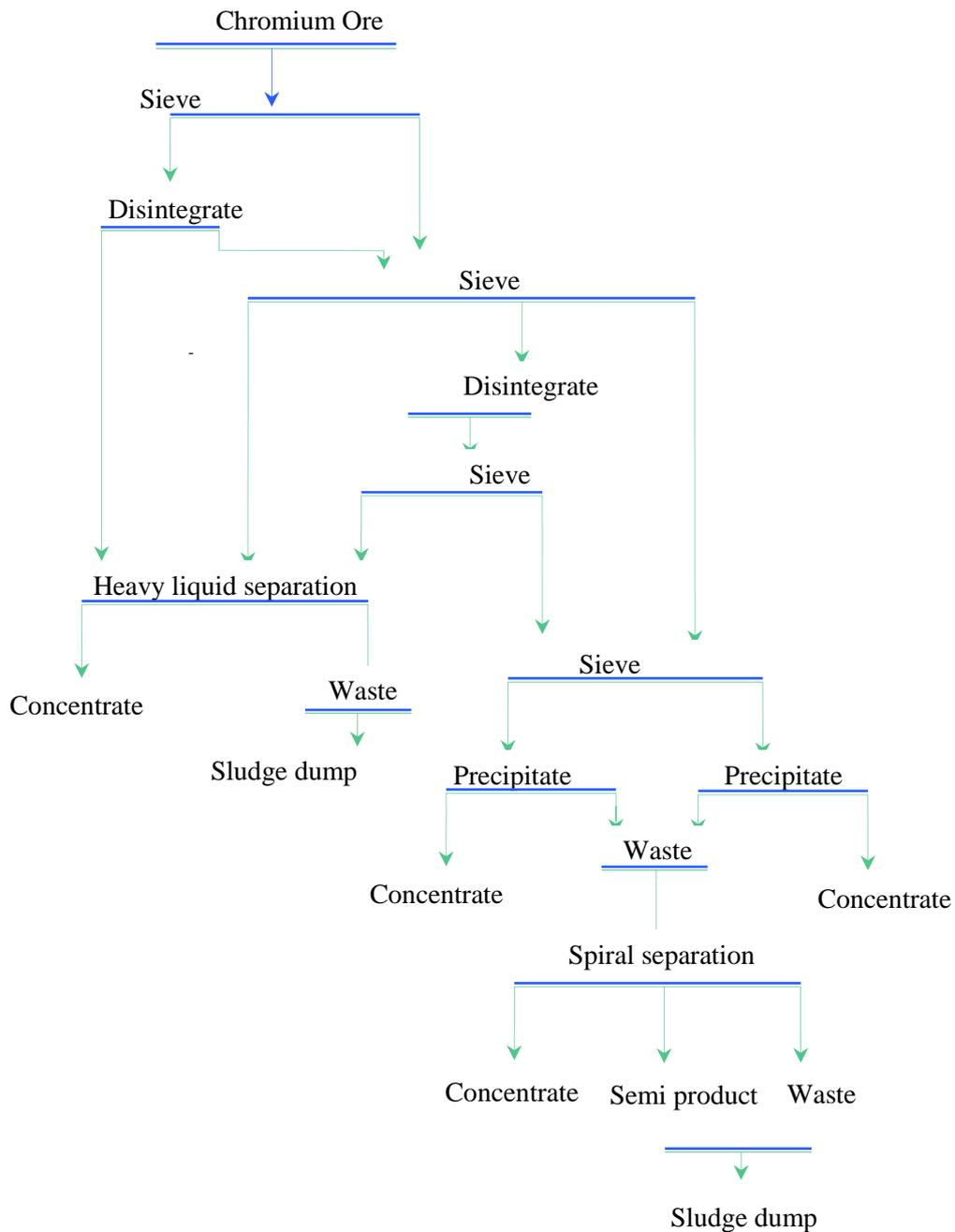
Figure-1. Scheme of DONSKOY'S ORE PROCESSING PLANT processing technology
